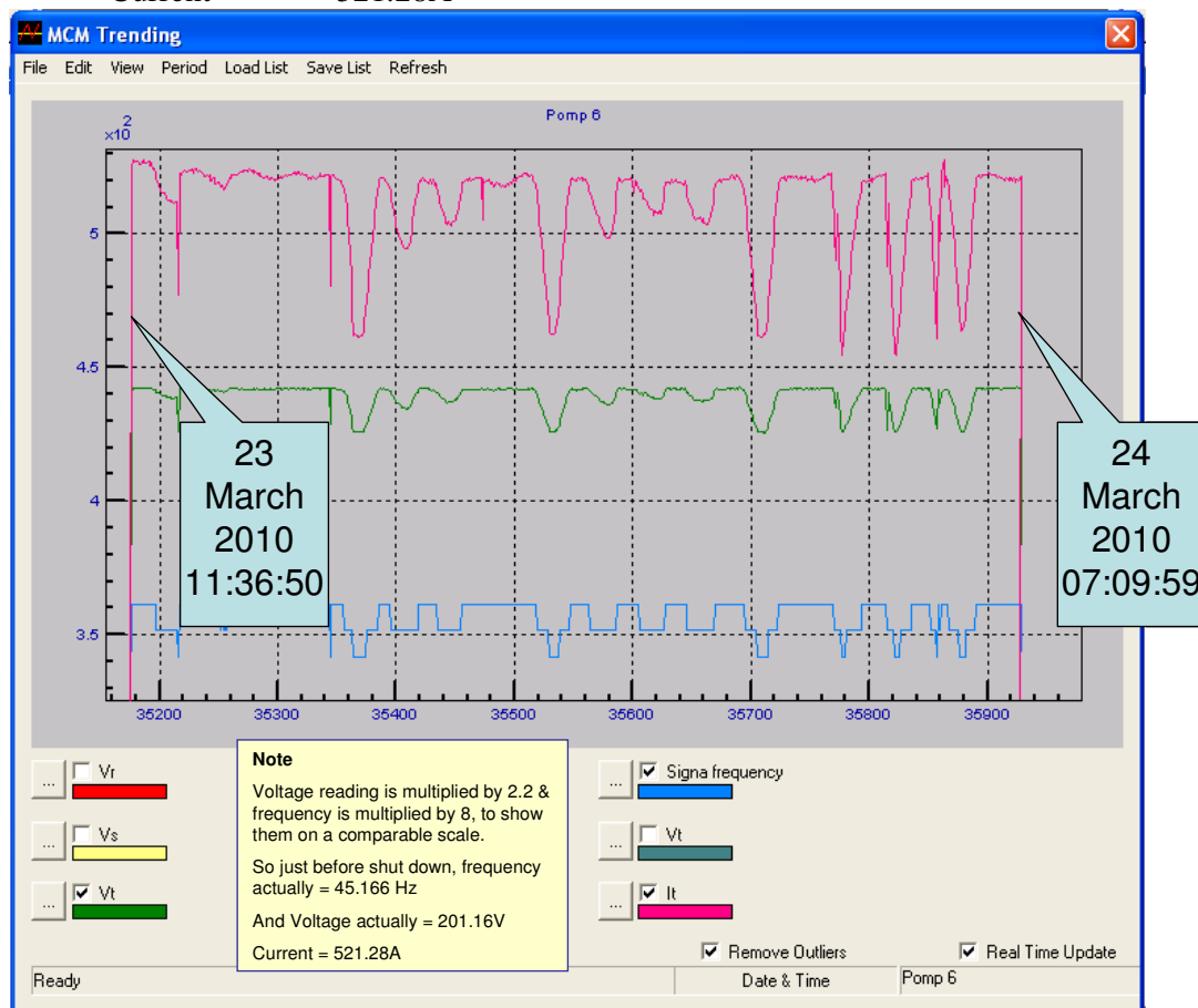
Figure 10: details of Voltage, Currency and Frequency of Drummer Road Pump 6 just before shut down on Wed 24 March.
