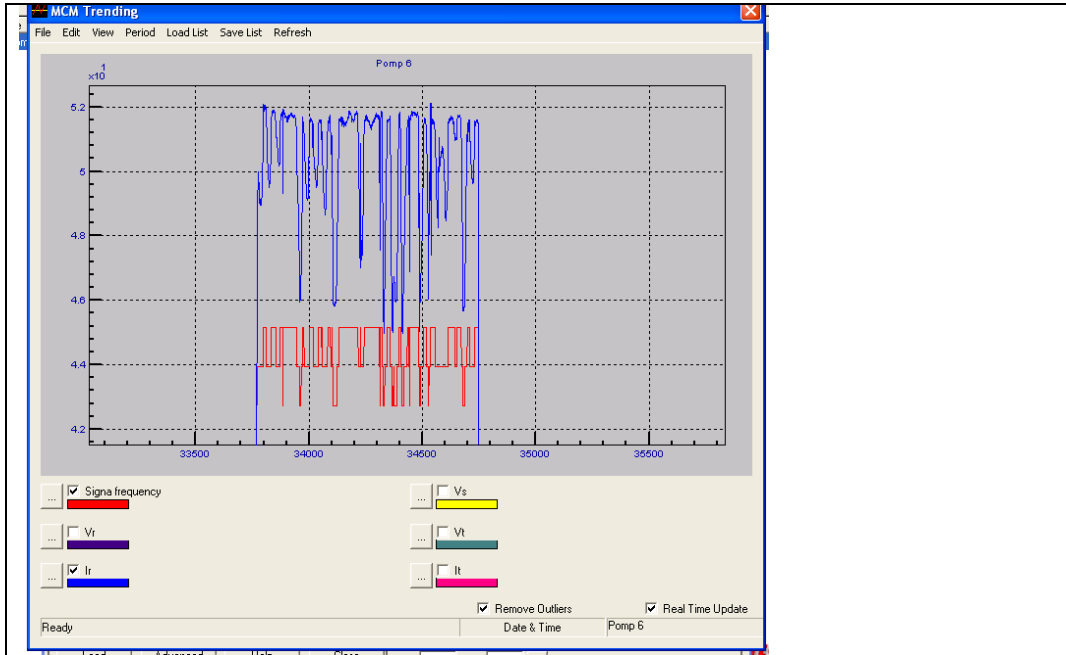
Figure 2: Motor Current and Frequency showing both within acceptable limits
